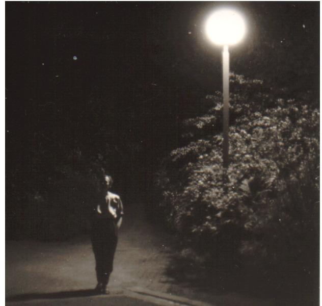
Figure 3 : Opaline-type luminaire with translucent envelope. The lamp-posts are at distances of 22 m maximum. Despite an average road illuminance or luminance level (0,5 to 1 \text{cd/m}^2 ), recognition is hardly feasible.
