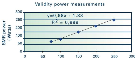
SMR power meter validation. SMR power was related to power delivered to the rear wheel by the velodyne, by the following equation :
