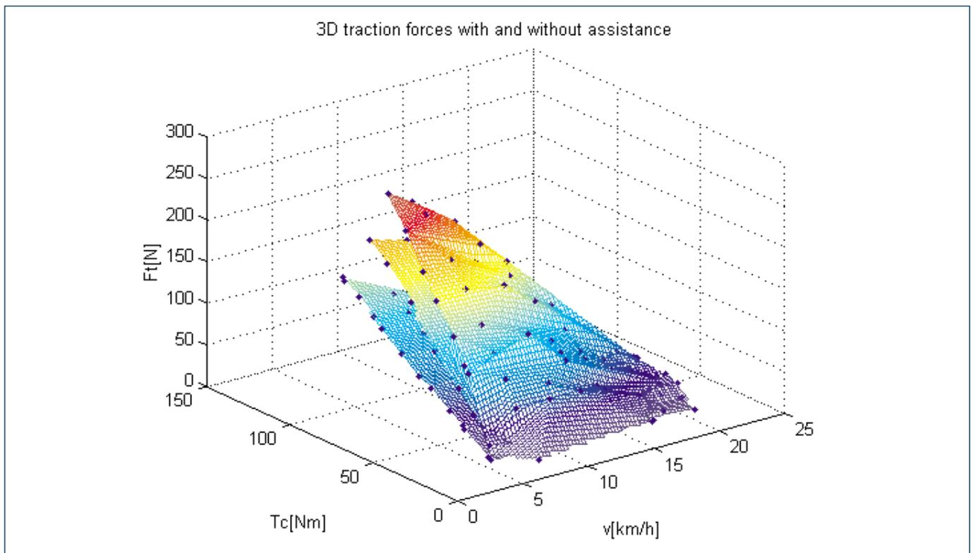
The measurements on the test bench confirm and quantify the driving comfort experienced on the electric bicycles. The mechanical efficiency of the tested EPACs, measured with assistance switched off, is significantly lower, however, than that of a normal bicycle.
